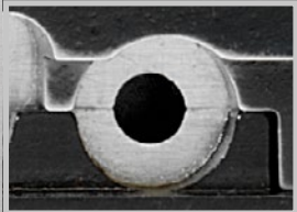
Stripping Area (Round Blades, no wire damage)
