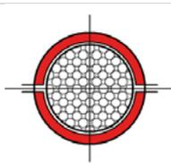
The shaped blades cuts the insulation completely. (The red area will be cut, no damaging of the cable strands)
