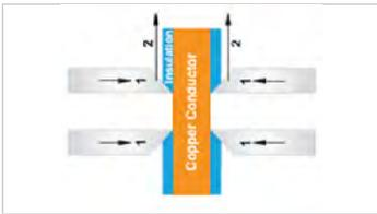
Two pairs of blades (1) cut the insulation to complete extent. Then the blade pairs move apart, and thus the insulation is removed form-fit (2). The pliers opens automatically after the stripping procedure.
