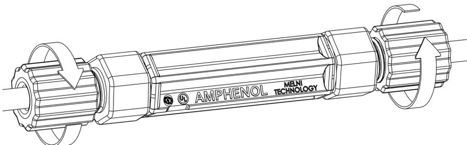
4.4.3. Using a Calibrated Torque Wrench and either a 3/4" or 20mm crows foot adapter, tighten BOTH of the Ratcheting End Caps to the EXACT specified torque shown in the table below. Or using wrench tool AMPVTW0001 to tighten the two Ratcheting End Caps.
