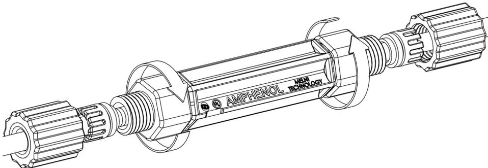
4.4.2 Re-install Sealing Gland, Collet and Sealing Caps. Lightly tighten the Sealing Caps by hand.
